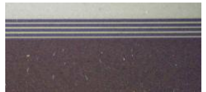
Ceramic laminate. The white outer layers have a thickness of \sim 50 \mu\text{m} .
