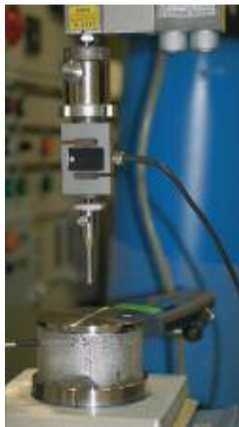
Lifetime test on piezo-electric sensor element under humid operating condition.
