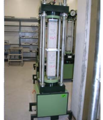
Figure 2: Testing device to apply a constant load over time (creep)
