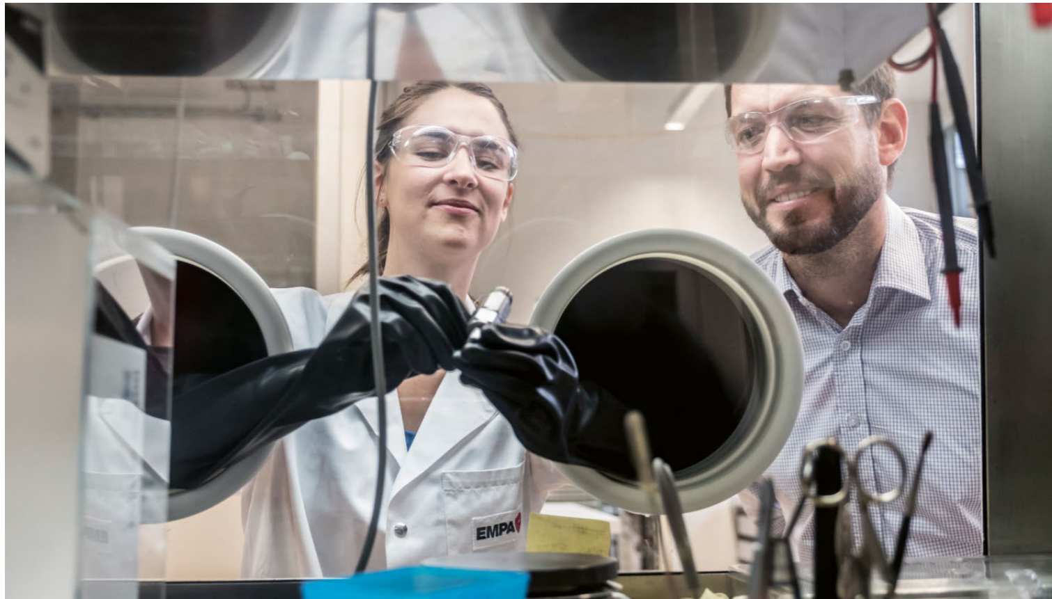
Where the prototype of a new battery is born: Marie-Claude Bay and Corsin Battaglia work in a "glove box" as the components need to be shielded from oxygen.
