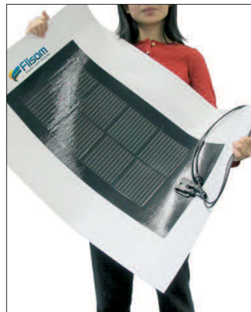
The flexible polymer solar cells, jointly developed by Empa and Flisom AG, a spin-off of ETH Zurich, were also a topic of discussion in the “Photovoltaics in Focus” seminar. (Flisom)
