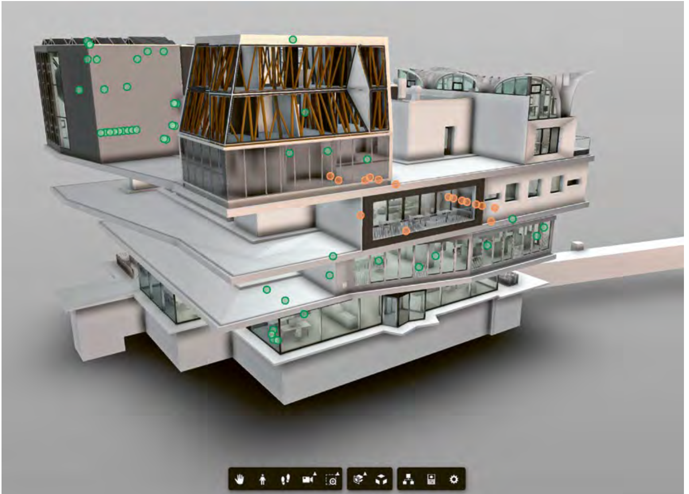
Live data in a 3D model: in the virtual NEST, the data from over 700 sensors and actuators are available in real time. Image: Dasher 360
