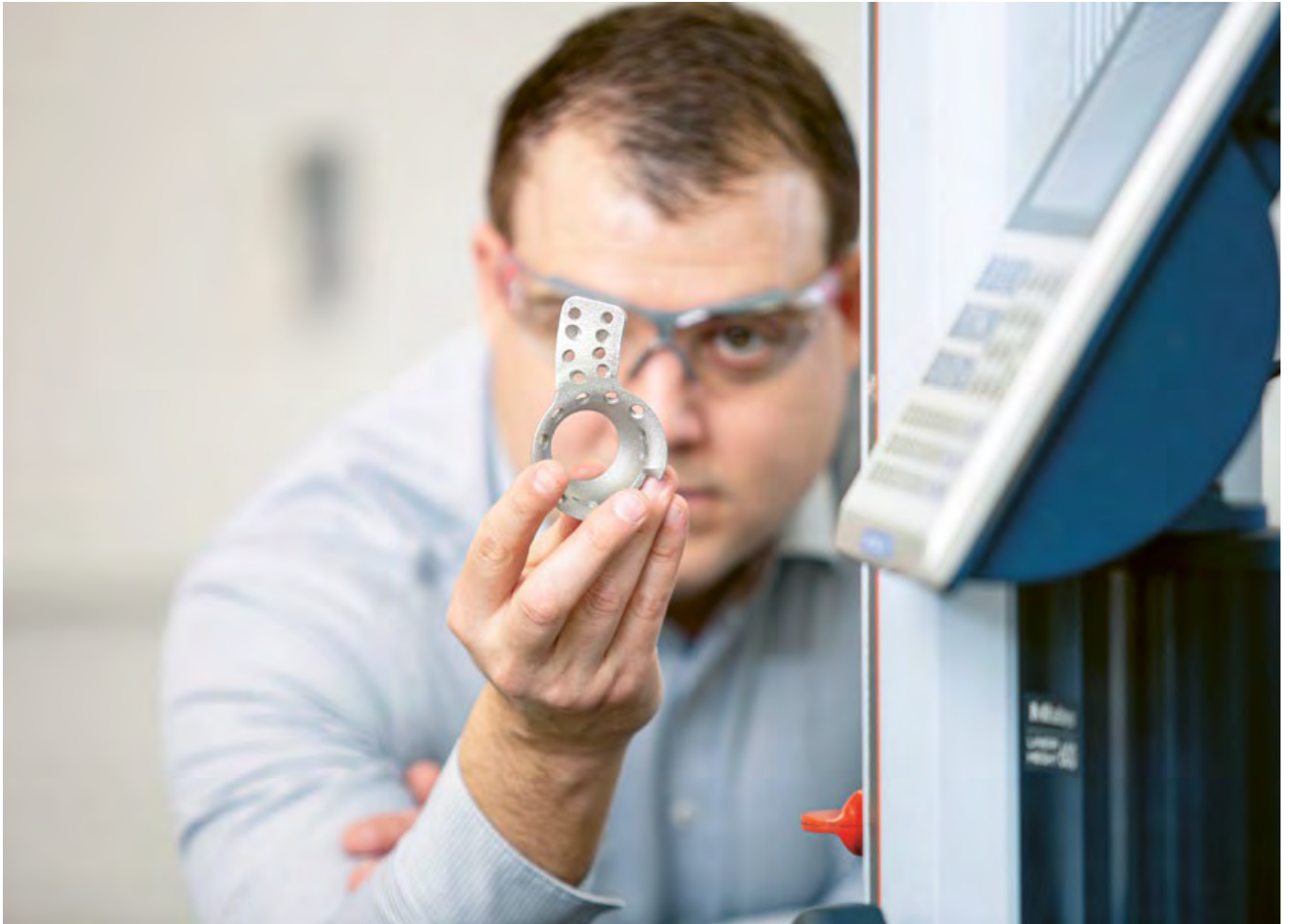
A 3D-printed reinforcement plate to hold an artificial acetabulum cup in case of complex pelvic fractures. (Photo: Swiss m4m Center)
