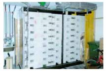
Above: Concrete formwork for the small batch production of the storage elements, spring 2015. The concrete storage system comprises 24 separate blocks, which were cast at Empa using a special concrete. Every block weighs around 400 kg and is streaked with copper piping. The blocks are placed in an insulated, watertight metal casing. The local plumber connects it up to the central heating.
