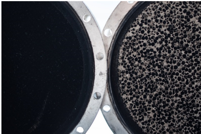
The tried and tested vs. the new and innovative: a monolithic catalyst (left) and a Foamcat (right).
