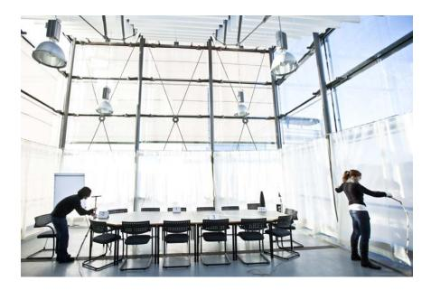
Acoustic tests using the sound-absorbing curtain were conducted in a typical meeting room at Empa: the reverberation time was measured using a loudspeaker and a microphone.
