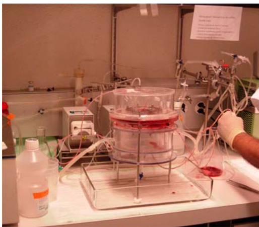
Ex-vivo placental perfusion system: In the perfusion chamber, the heart of the device (centre), blood flow is maintained in the maternal and foetal circulation zones of the placenta, keeping it viable for several hours after birth.
