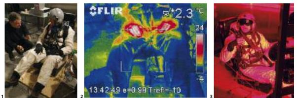
pulse pilots, accumulations of moisture can become an especially serious problem because the seat in the aircraft covers a third of their body surface. In order to also purge moisture efficiently from the seating regions, Weder and his team incorporated active rear ventilation into the pilot's seat and the areas of the suit covering his back.
