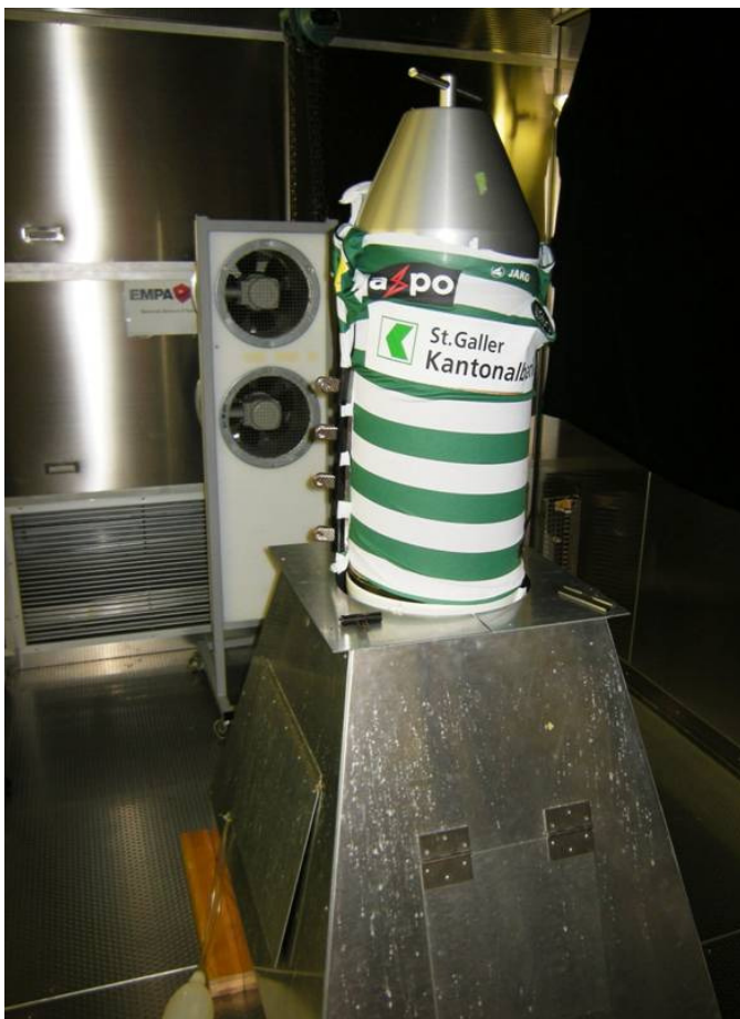
Measuring the rate of humidity transport with liquid perspiration on the test torso in a climate chamber at Empa.
