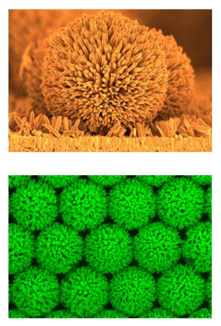
«Sea-urchins» made of tiny polystyrene balls, with zinc oxide nanowire «spines» are created using a simple electrochemical process.
