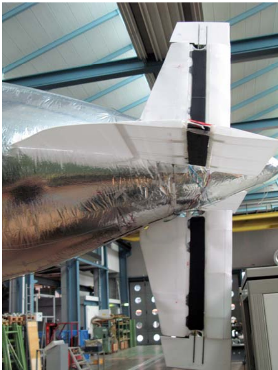
Electroactive polymers (EAPs) control the altitude and lateral movement of the current version of the Empa blimp. To this end, electrically activated elastic polymer films have been fitted as hinges in the blimp's fin assembly (black). (Photo: Empa)
