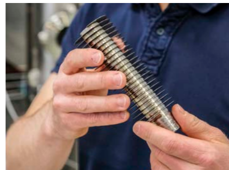
Heat exchangers from instant water heaters provided the solution: the sodium hydroxide solution spirals along a pipe, absorbs water vapor and emits heat.
