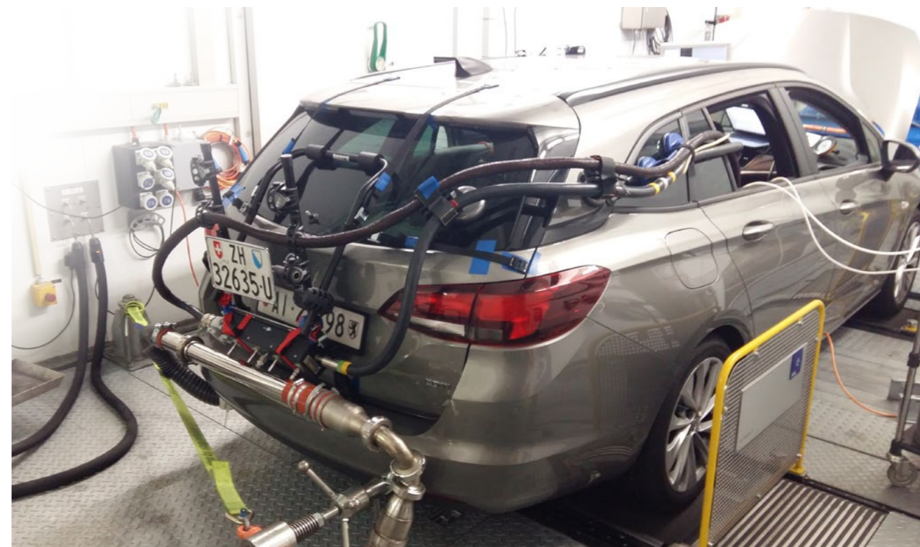
An Opel Astra 1.6 CDTI on Empa's dynamometer test rig: the tubes connect the exhaust tract to a mobile PEMS device (portable emission measuring system) inside the car. Thus equipped it then heads off around Lake Greifensee.
